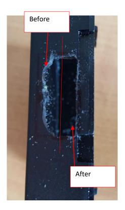
Keep testing too see if the switch will fit into the hole. If it is tight keep filing.
