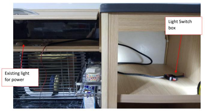
**Step 9**Remove any covers to where you will be tapping into for the 12volt power.
