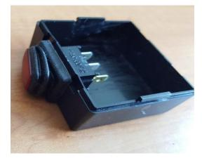
**Step 6**Place the back cover into position
